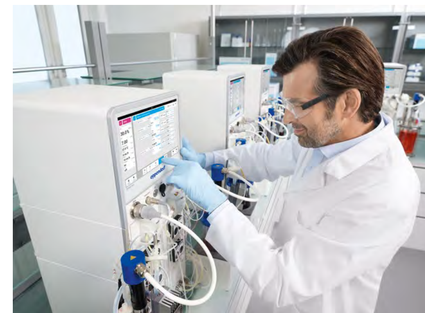
VisioNize®-onboard software on the 12 in touch display with ultra wide view angle, integrates the SciVario twin into the Eppendorf digital lab
